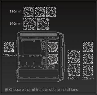
Two big frontal vents with detachable filters guarantee a clear air intake, while two side vents on both sides of the top cover create an excellent way for the exhaust to leave the case without dust getting in.
