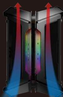
Two elongated chambers, with up to five fans and a massive lateral vent each, provide your components with an uninterrupted and potent airflow that will keep components' temperatures under control while the cable management space between the two chambers allows heat to dissipate. For extra cooling in the primary chamber, it supports up to two 240mm radiators.
